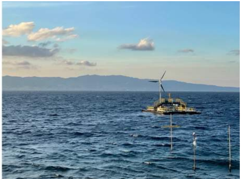
The large-scale wind turbine model installed on the multi-purpose platform and deployed in front of NOEL laboratory (Reggio Calabria, Italy) for the experimental campaign of "The Blue Growth Farm" EU H2020 project.
