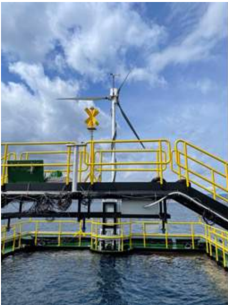
The large-scale wind turbine model installed on the multi-purpose platform and deployed in front of NOEL laboratory (Reggio Calabria, Italy) for the experimental campaign of "The Blue Growth Farm" EU H2020 project.
