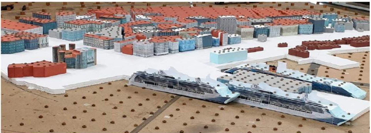
The reduced-scale physical model of the port of Naples realized in the wind tunnel
