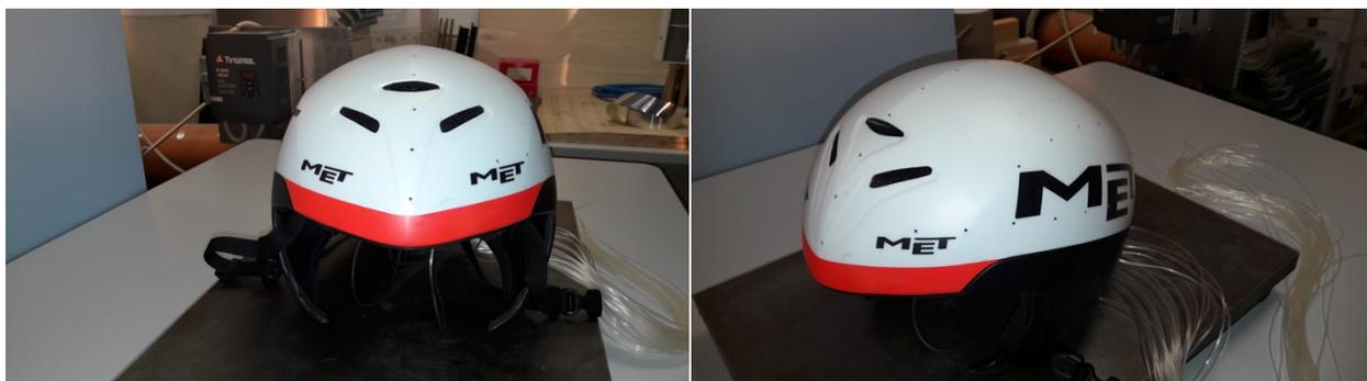
Figure 3. Instrumented helmet for pressure measurements
