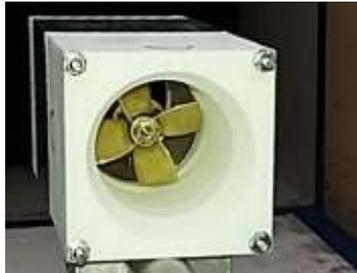
Figure 1 Rotor placed in the duct
