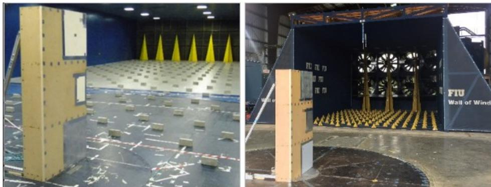
Figure 1: test section of PoliMi wind tunnel (left) and WoW wind tunnel (right).
