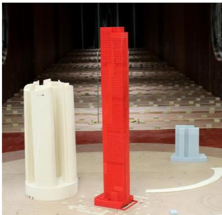
Figure 1 - Original model in the wind tunnel
