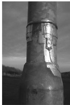
Fig. 1. Experimental lighting columns (a); strain gauges at the welded-joint (b).
