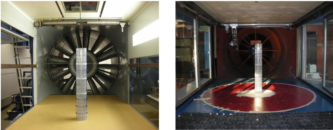
Fig. 1. Wind tunnel tests on Solar Updraft Tower. a) WiSt, Ruhr-Univ. Bochum, Germany; b) Criaciv, Univ. Florence, Italy
