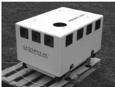
Figure 2.13 Small pulsed Doppler wind LIDAR for measurement of wind profiles in a height range between 40 and 200 m. Distance determination by pulse travel time (Emeis, 2010)
