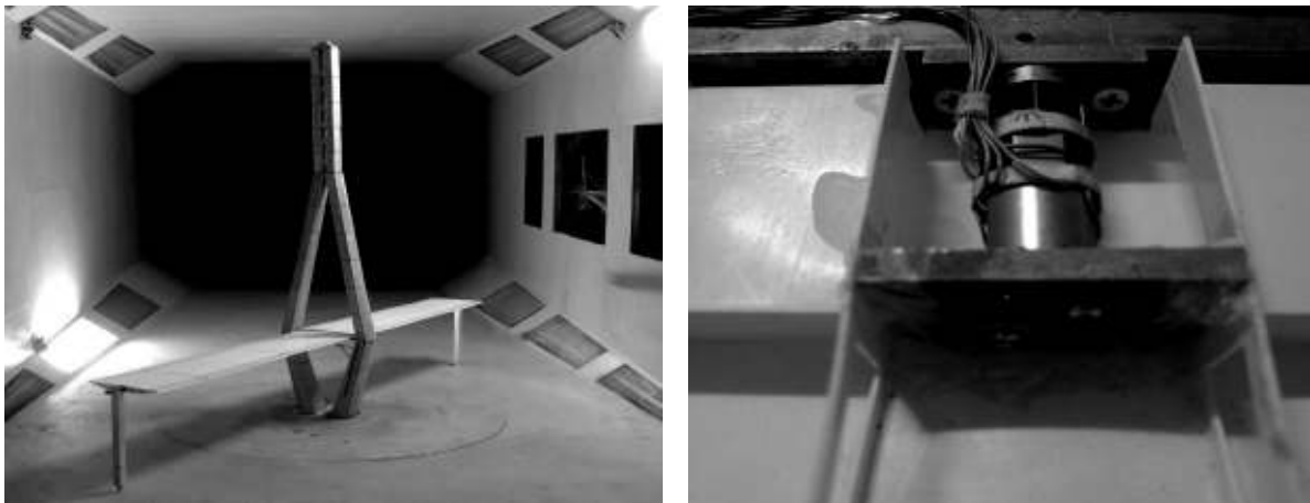
Figure 1. Full bridge aero-stiff model of a cable-stayed bridge (left) and force balance inside deck segment (Right)
