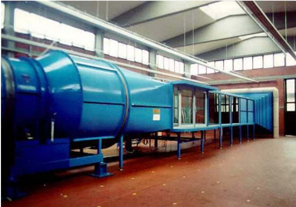
Fig. 6.1 View of the CRIACIV-DICEA Boundary Layer Wind Tunnel in Prato.
