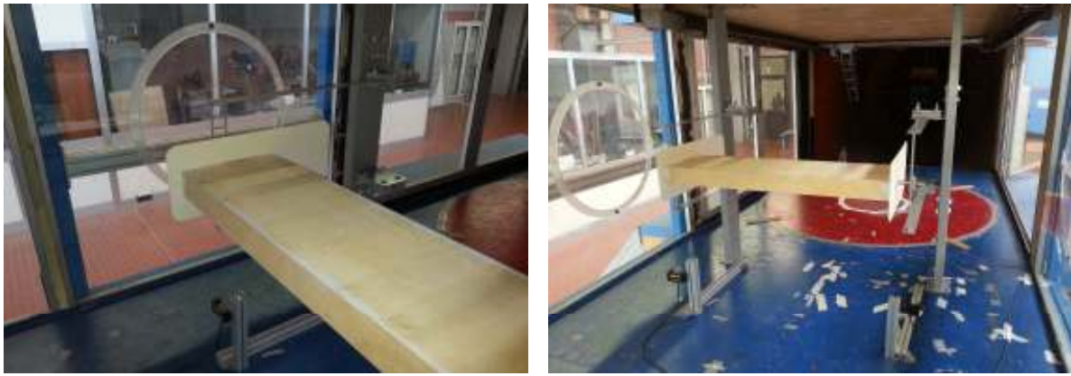
Figure 1. Experimental set-up: sectional model (left), suspension system (right).
