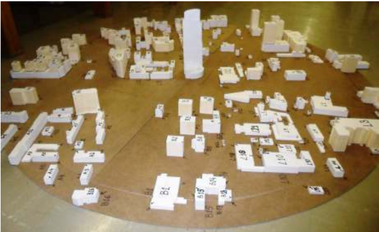
Figure 7. Surroundings model used for wind-tunnel tests.
