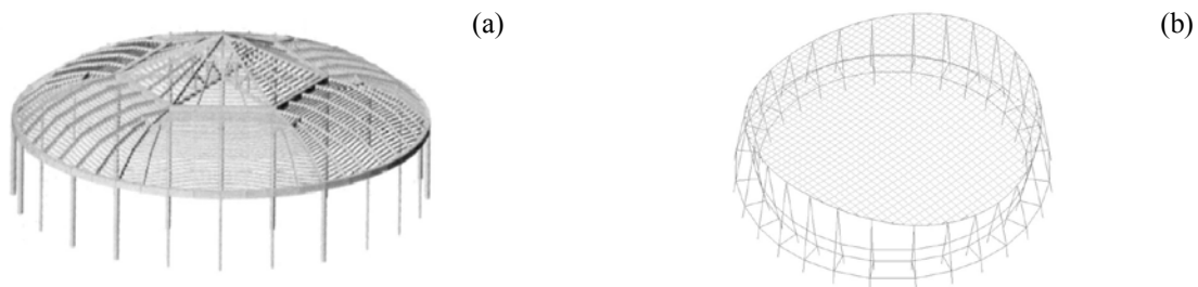
Figure 12. CS1 (a) Glued laminated timber roof -approved project- (b) HP Cables net roof -alternative proposal-
