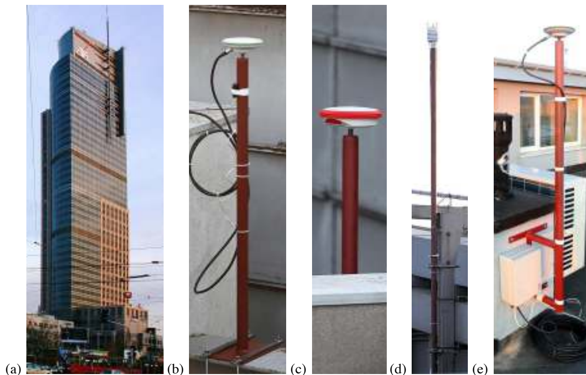
Figure 1. Warsaw Trade Tower building (a) and full-scale measuring equipment: RTK-GNSS rover stations (b, c), weather station (d) and RTK-GNSS reference station (e).
