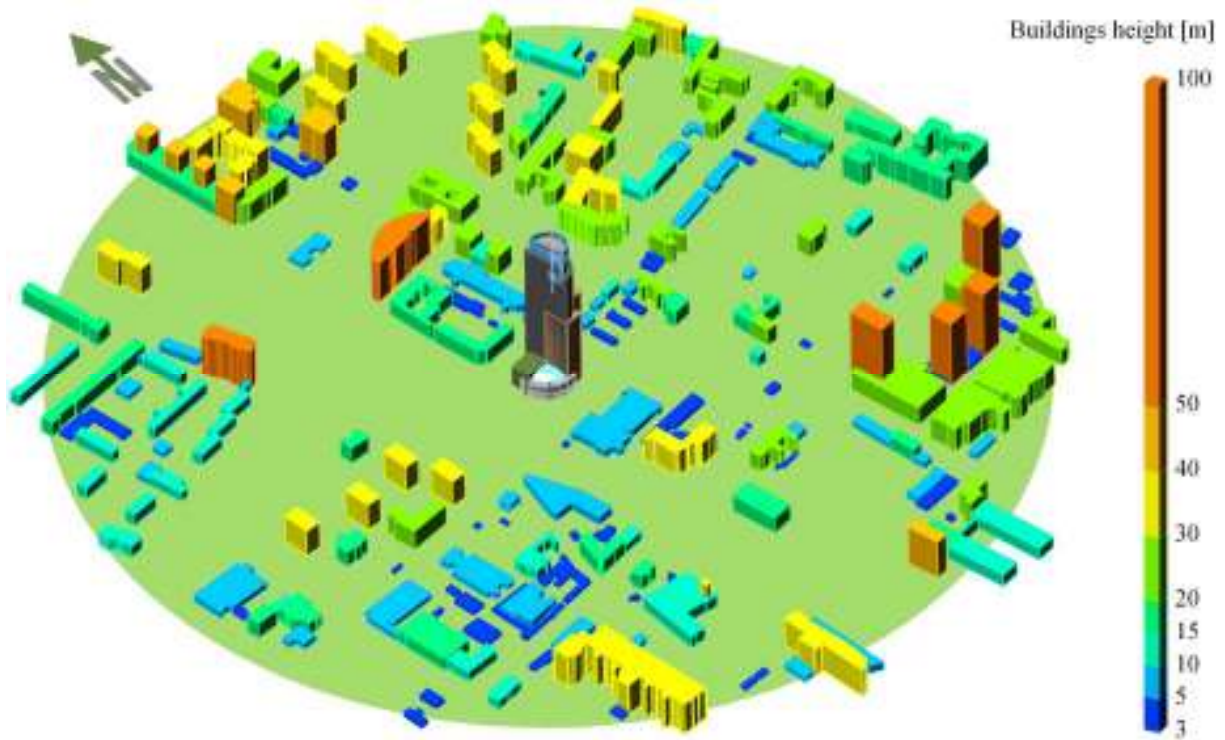
Figure 9. 3D digital WTT building and surroundings model – central section of the computational domain.
