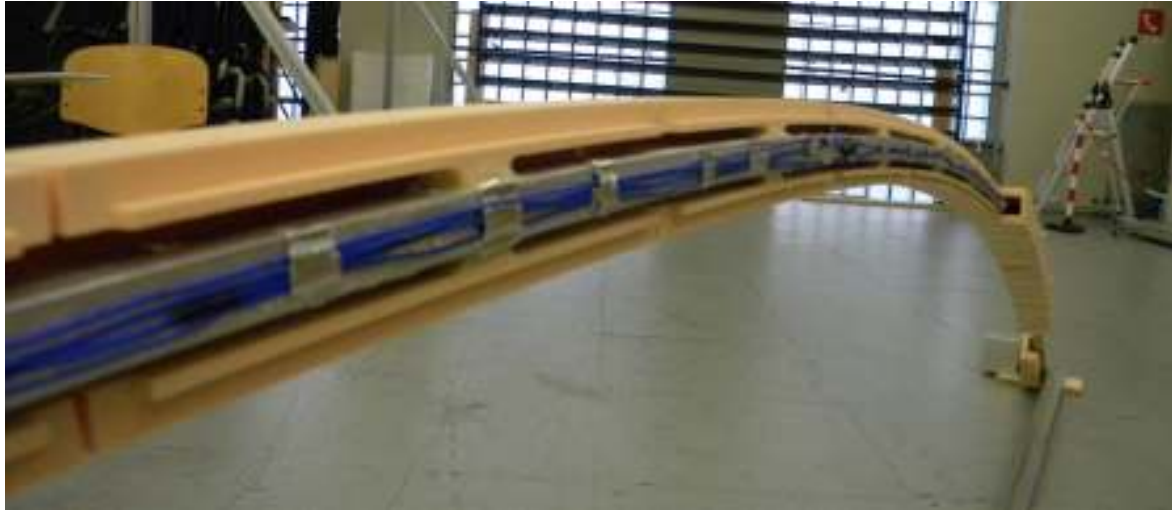
Figure 1. Full aeroelastic model of the Arco while building it. The connection between the external shells and the spine are clearly visible.
