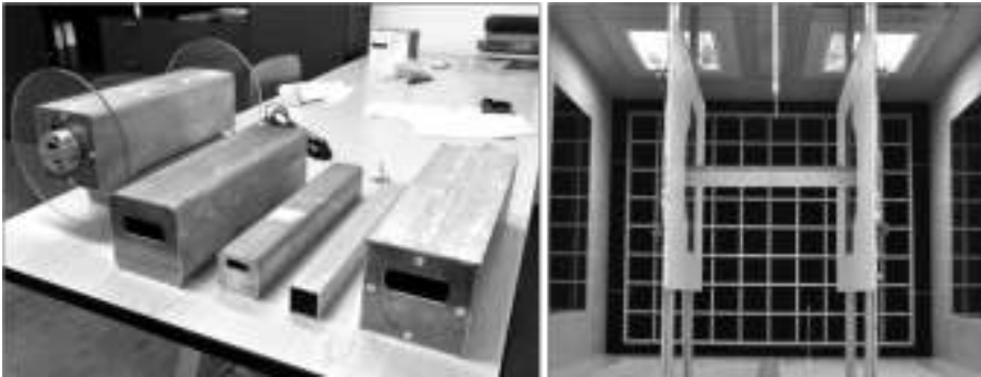
Figure 7.1 Wind tunnel, experimental setup: tested models (left) and turbulent flow condition by wood grid (right).
