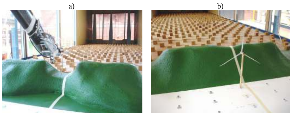
Figure 1. Experimental setup in the wind tunnel test section: a) castellated barrier wall, vortex generators, surface roughness and the mountain with a bay model, b) the offshore wind-turbine model placed 5 cm downstream from the trailing edge of the large mountain model.
