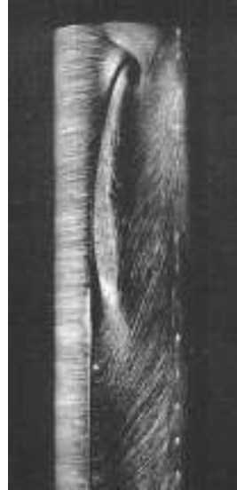
Figure 3.22 Flow pattern in the tip region: a) Sketch of tip trailing vortices (ESDU 96030); b) Flow visualization at high Re (Gould et al., 1968);
