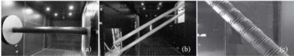
Figure 2.1. Wind tunnel test on a plain cable (Matteoni and Georgakis, 2012) (a), a filleted twin-cable (Mattiello et al., 2013) (b) and a new cable surface modification (Kleissl and Georgakis, 2012) (c).
