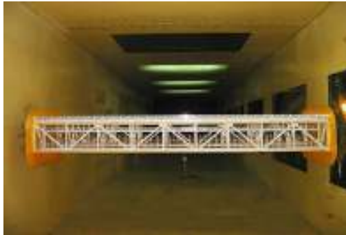
Figure 11 Section Model of Baling River Bridge
