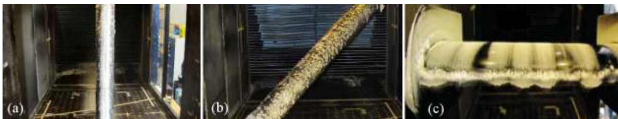
Figure 2.2. In-cloud ice accretion on a bridge hanger (a), and on a stay cable (b) (Demartino, 2014) and on a wind turbine blade (Hudecz et al., 2013) (c).
