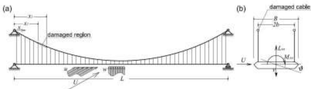
Figure 1. Continuum model of suspension bridge with damaged main cable (a), lift and pitching moment per unit length acting on the deck (b).
